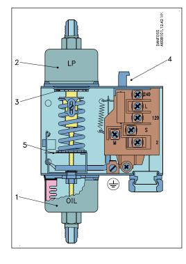
The operation of the pressure control is based only on the differential pressure, i.e. the difference in pressure between the two counteracting bellows, whereas it is independent of the absolute pressure acting on both bellows.
