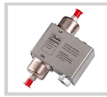
MP 54 and MP 55 oil differential pressure controls are used as safety switches to protect refrigeration compressors against low lubricating oil pressure.
